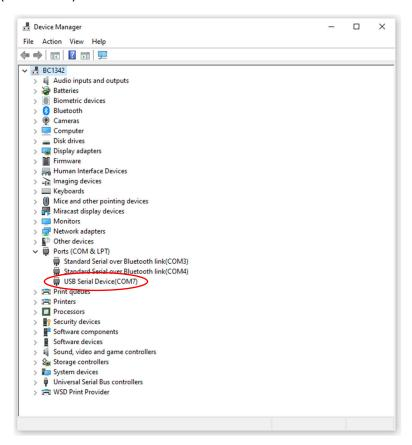
D. Open u-center and click ▼ to open the port connection and select the USB port for the GPS.
